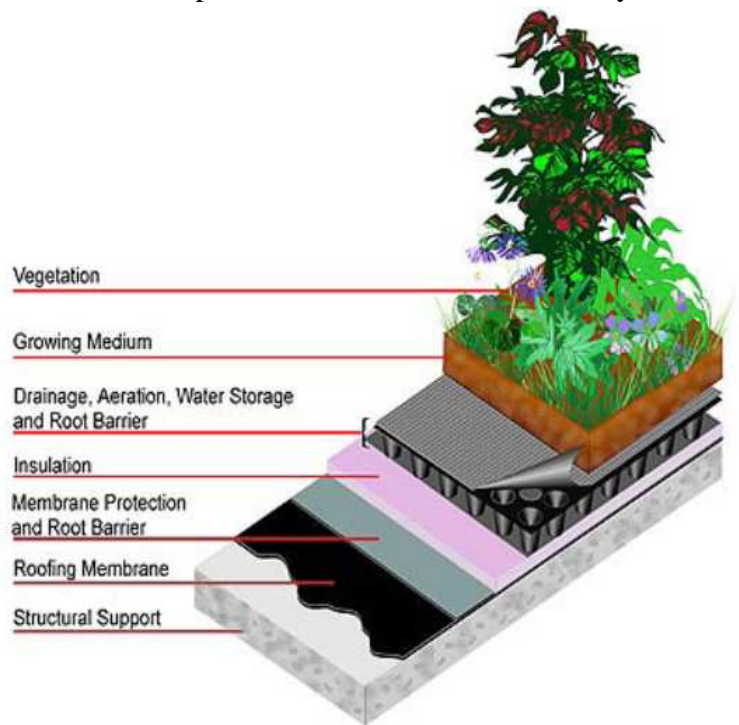
Figure 1: Structure of a Green Roof (Source: heatusa.com)
